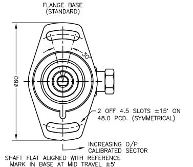
0.5 TO 4.5V RATIOMETRIC SUPPLY CURRENT 12mA TYP. 20mA MAX. CABLE: 0.2mm², O/A SCREEN, PUR JACKET — SUPPLIED WITH 50cm OR REQUIRED LENGTH IN cm (15000cm MAX). STANDARD 3—CORE: JACKET Ø4mm BLACK e.g. 'L50' OPTIONAL 5-CORE: JACKET Ø4.6mm BLUE e.g. 'LQ50' CABLE/CONNECTOR\* CONNECTIONS; 3 CORE 5 CORE CONNECTOR RED ORG :1
